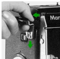
While pushing in on the rear blade of the neck strap fastener with your thumb, slide it in the direction opposite to that for attaching, and remove the fastener.
